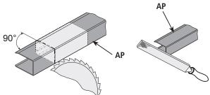
■ Check the swivel area of the drive and if necessary cut out the cover profile AP in the area of the brackets.
