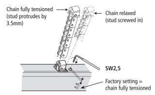
Always note the force-path diagram (see chapter "Data sheet KSA-Twin S12 24V") and rigidity of the chain, depending on the installed position!
