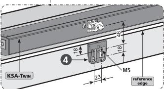
■ Slide casement bracket **F44 3** on the baseplate **4** and secure with screw **5**.
