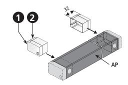
■ If necessary, feed the cable through the hole in the end cap or close off the hole with blind plugs ④.
