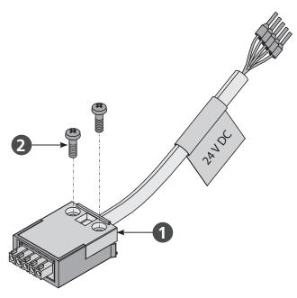
Note Locking hooks - at the housing cover • prevent withdrawal of the plug under tensile load.
