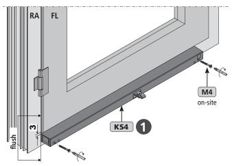
■ Fix and align the casement bracket **F55 ②** onto casement (**M5**) (insert rivet nuts on-site). See the drawing "Drilling dimensions for drive KS4 and casement bracket F55" on the previous page.
