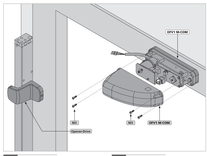
The window must be closed before the assembly.
