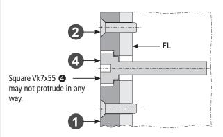
■ Insert the locking drive **OFV1 M-COM** into groove of square Vk7x55 **4** and fasten it with two screws **5** and spring rings **6** on the adapter plate **1**.
