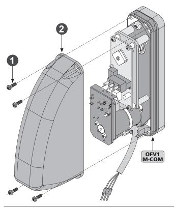
■ Using the screws **1** and mount the housing **2** on the locking drive **OFV1 M-COM**.
