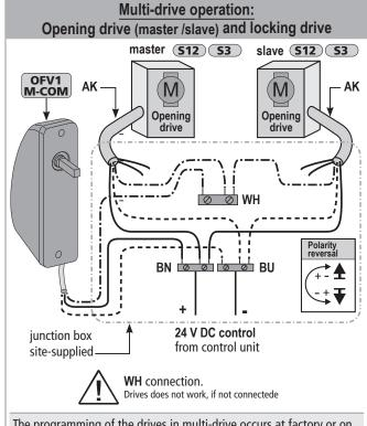
The programming of the drives in multi-drive occurs at factory or on site with Parameterisation-Interface
