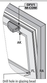
Drill hole in glazing bead (cable bushing protects against damage to cable).
