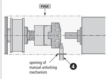
Note Cross-head screw driver Phillips size 3 4 is not included in the scope of delivery.
