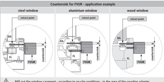
Mill out the window casement - according to on-site conditions - in the area of the coupling adapter.
