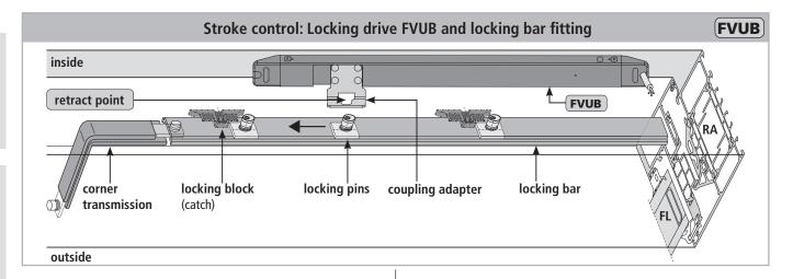
■ Screw locking drive **FVUB** onto window frame (**M5**).
