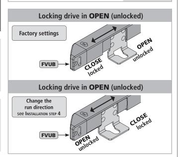
■ Check whether the stroke of the locking drive **FVUB** with the stroke of the on-site locking bar moves synchronously.
