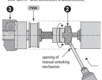
■ Insert a cross-head screw driver Phillips size 3 **4**- through opening of unlocking mechanism - into the groove of the gear wheel **2** (bevel pinion).
