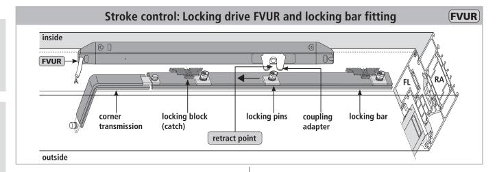
■ Screw locking drive **FVUR** onto casement frame (**M5**).
