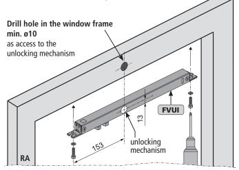
■ Carefully punch through the sticker **①** of the unlocking mechanism.
