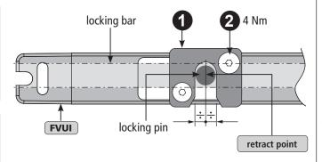
■ Mount the locking drive **FVUI** with screws **3** and washers **4** in the pre-cut (milled out) window frame.
