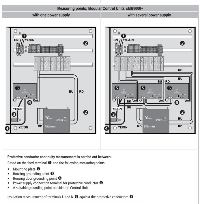
The residual voltage measurement on the power supply: Terminal L against terminal N  $\textcircled{\mbox{\sc o}}$
